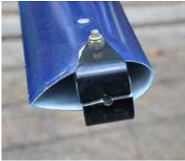
Figure 4. Fractured right front lift strut bracket
