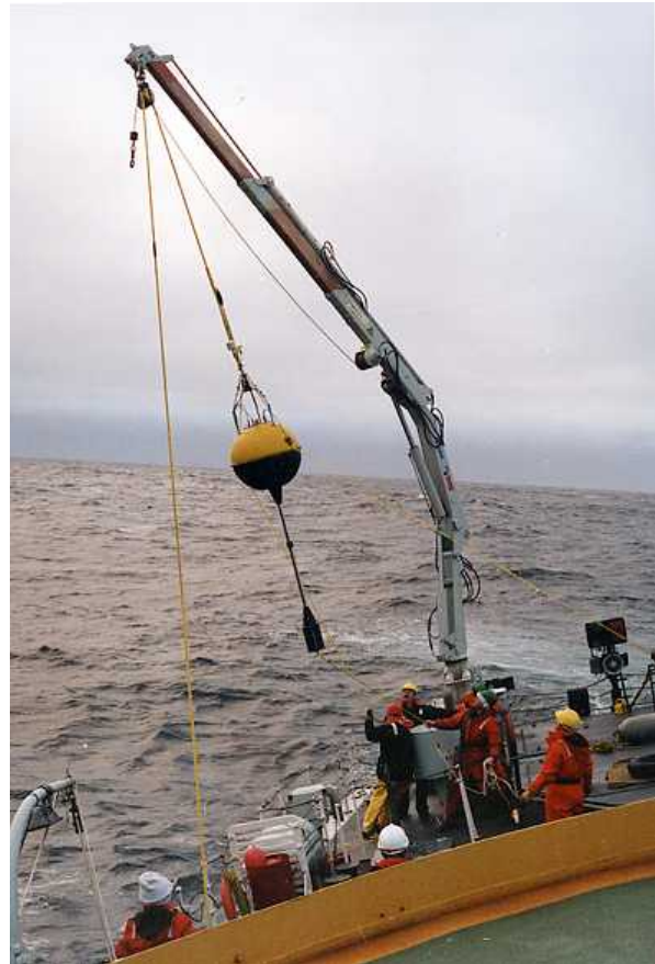
Figure 3: Endeco Wave Buoy Being Deployed from HMCS Nipigon
